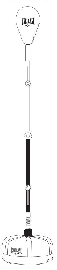
ATTENTION: Do not operate with both springs fully locked or unit may be damaged. Each spring lock needs to be at the top or bottom position. Do not lock in middle or unit may be damaged. Do not operate otherwise or unit may be damaged. Do not unscrew and remove the lock knobs.
